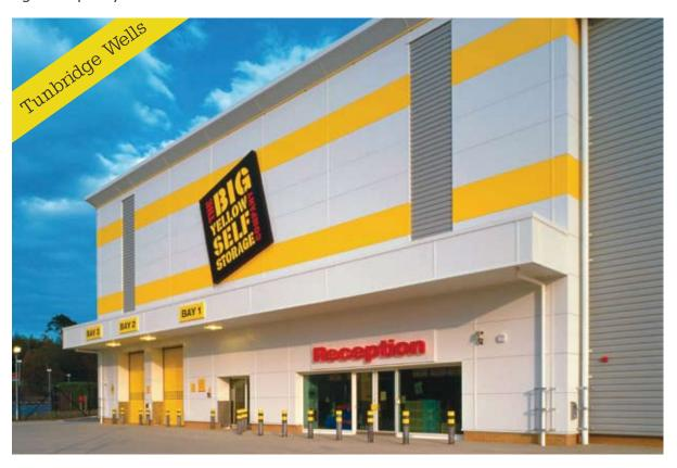
Big Yellow Self Storage, Tunbridge Wells like other store in the portfolio has materials with a high recycled content including aluminium window frames, particle board flooring (recycled bark and sawdust), blocks (recycled pulverized fuel ash) and Rockwool solid insulation (recycled slag)
